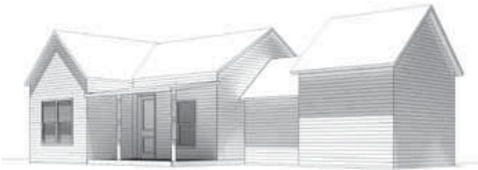
*The Design Guidelines specifically show how a transitional element, or connector, differentiates the new addition from the historic house (page 34).*
