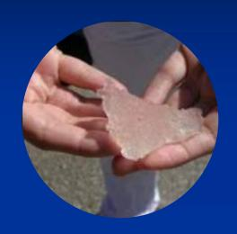
To maintain the correct consistency of the Ice Pig during an operation a **freezing point depressant is used**
