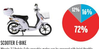
Wheels: 2 | Pedals: Fully operable; motor can be engaged with twist throttle Speed at which motor power stops: 20 mph | Weight: 165 lbs
