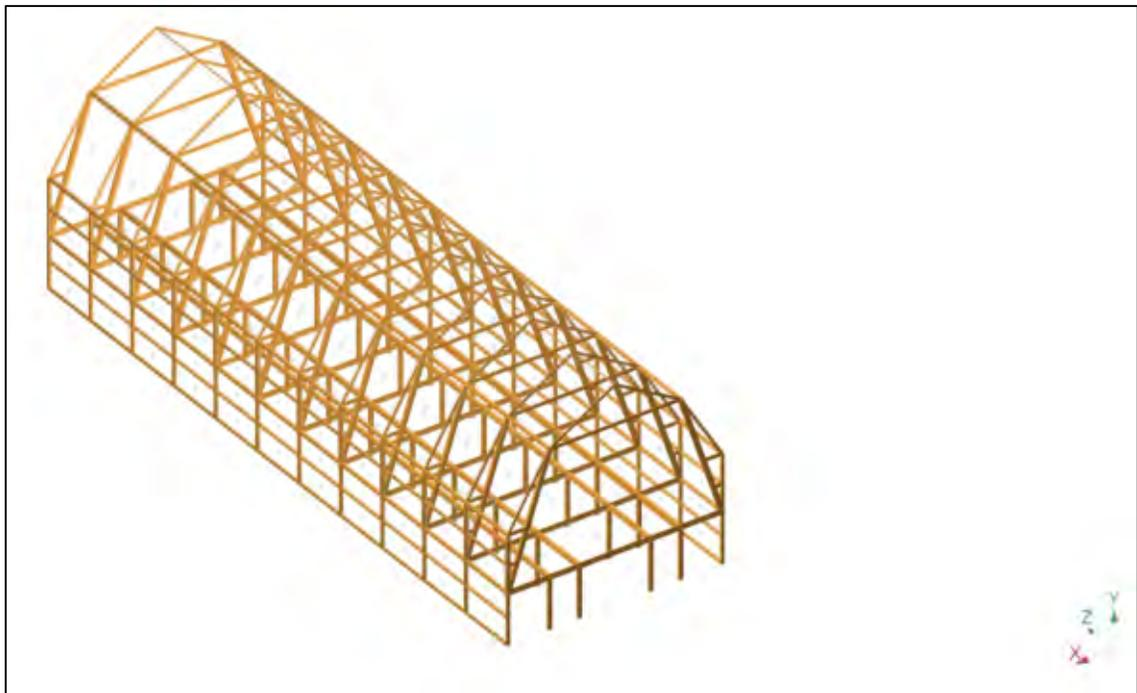
Figure 4. Computer Model of the "as-is" Barn Structure
