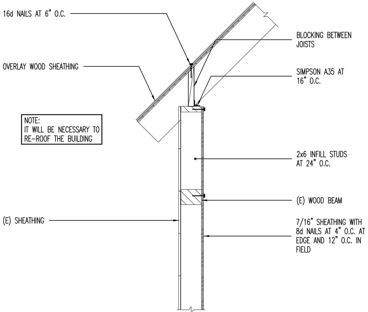
**5A** SHEAR WALL TO ROOF CONNECTION - OPTION A
