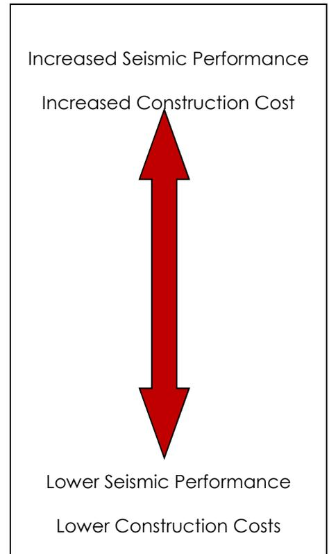
A building designed or retrofitted to an Operational Level would be expected to be fully functional with little to no damage following an earthquake. Meanwhile a building designed to a Collapse Prevention Level would only be expected to be stable enough to allow people to exit during a seismic event. The building may be a complete loss with damage beyond reasonable repair costs.
