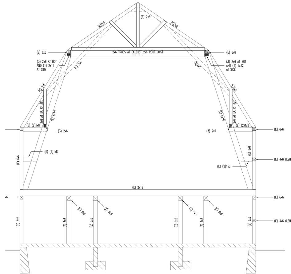
**A** BARN/TRUSS SECTION ROOF RETROFIT
