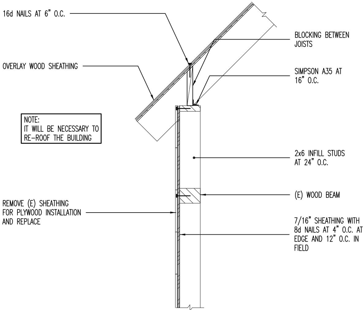
**5B** SHEAR WALL TO ROOF CONNECTION – OPTION B
