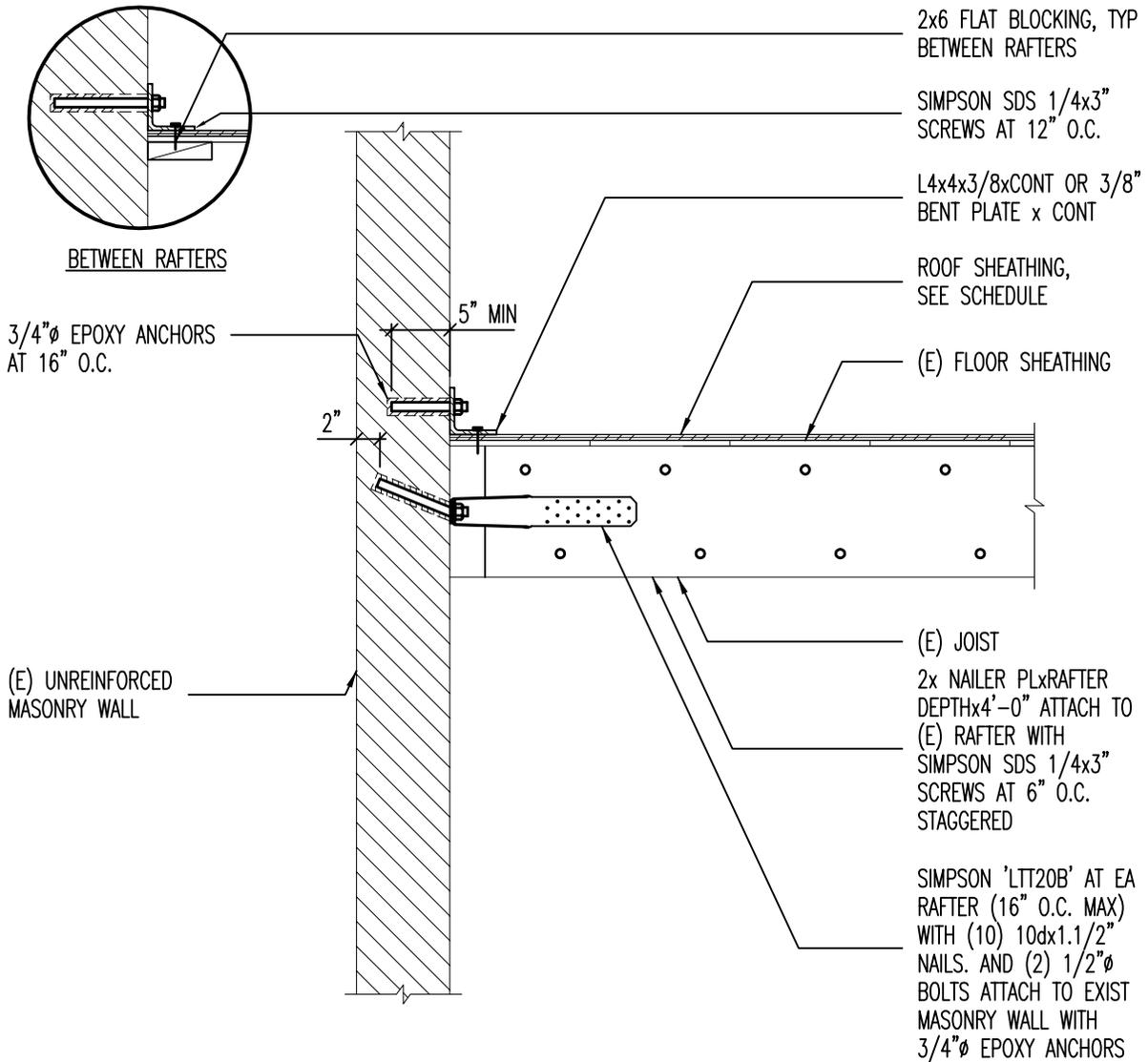
**6** TYPICAL FLOOR ANCHORAGE DETAIL AT URM
