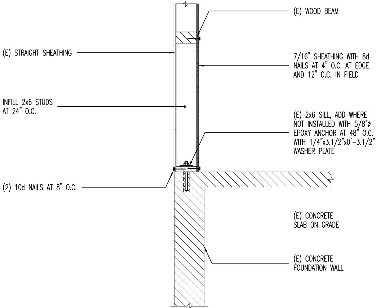
**3A SHEAR WALL TO FOUNDATION DETAIL OPTION A (DEFICIENCY 3c)**
