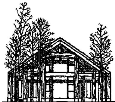
Fig 2-8: Large viewing windows shall be recessed under overhangs.
