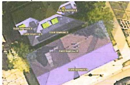
Relocation of the panels to the North East roof of you building is not a good option. Relocation of your panels would result in a 65% production loss. The cost to relocate the panels would not be offset by the panels production.
