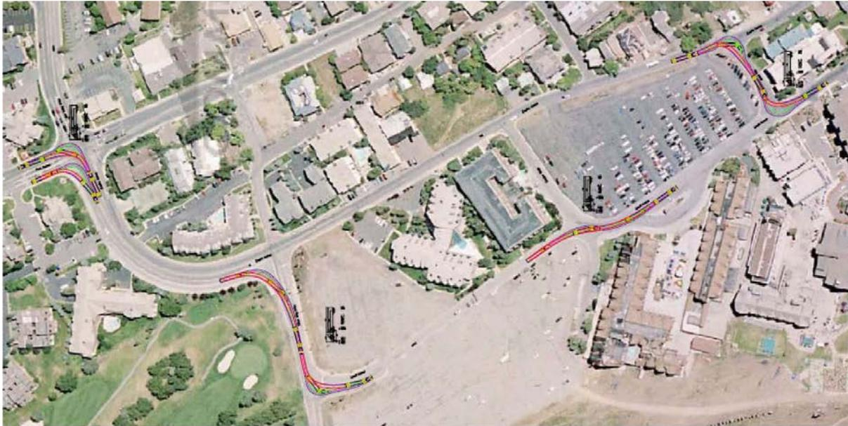
Overall view of the intersections evaluated for truck turning templates
