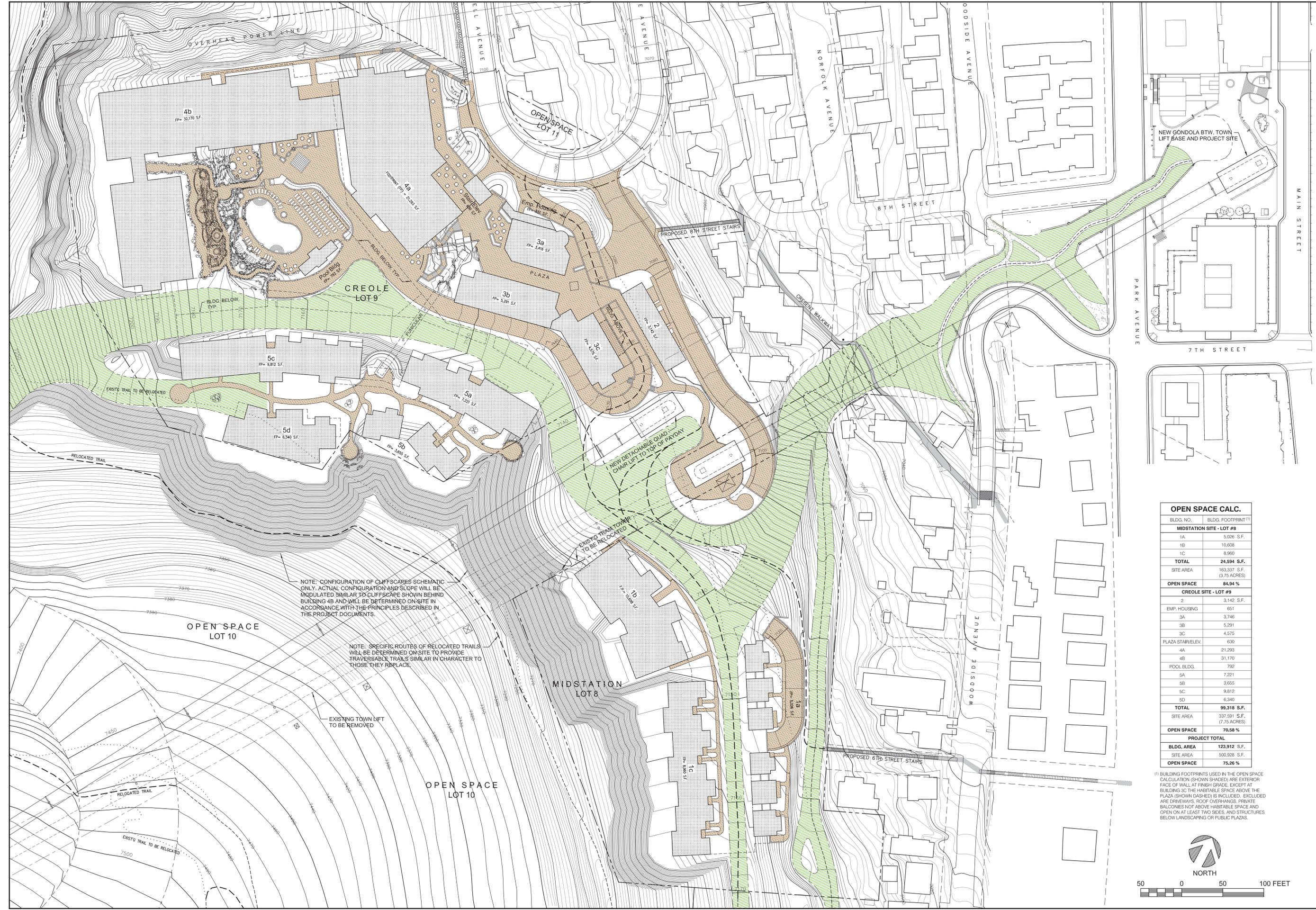
NOTE: CONFIGURATION OF CLIFFSCAPES SCHEMATIC ONLY. ACTUAL CONFIGURATION AND SLOPE WILL BE MODULATED SIMILAR TO CLIFFSCAPE SHOWN BEHIND BUILDING 4B AND WILL BE DETERMINED ON-SITE IN ACCORDANCE WITH THE PRINCIPLES DESCRIBED IN THE PROJECT DOCUMENTS.
