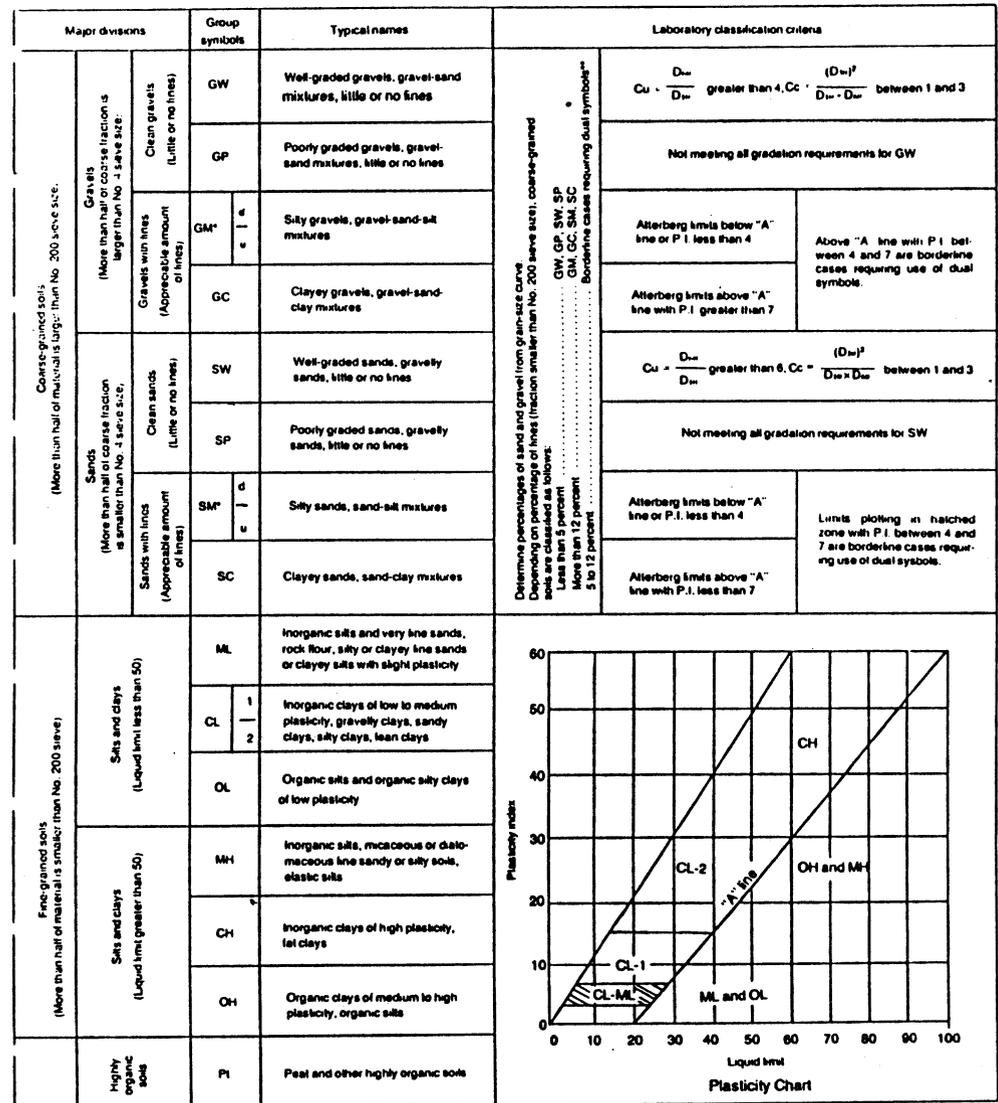
\* Division of GM and SM groups into subclasses of d and v for roads and airfields only. Subdivision is based on Atterberg limits, silt <math>L.L.</math> is 28 or less and the P.I. is 6 or less, the silt <math>L.L.</math> is greater than 28.
