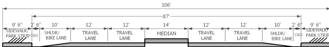
**Figure 28: Modified Seven-Lane Cross-section, 106' Right-of-Way**
