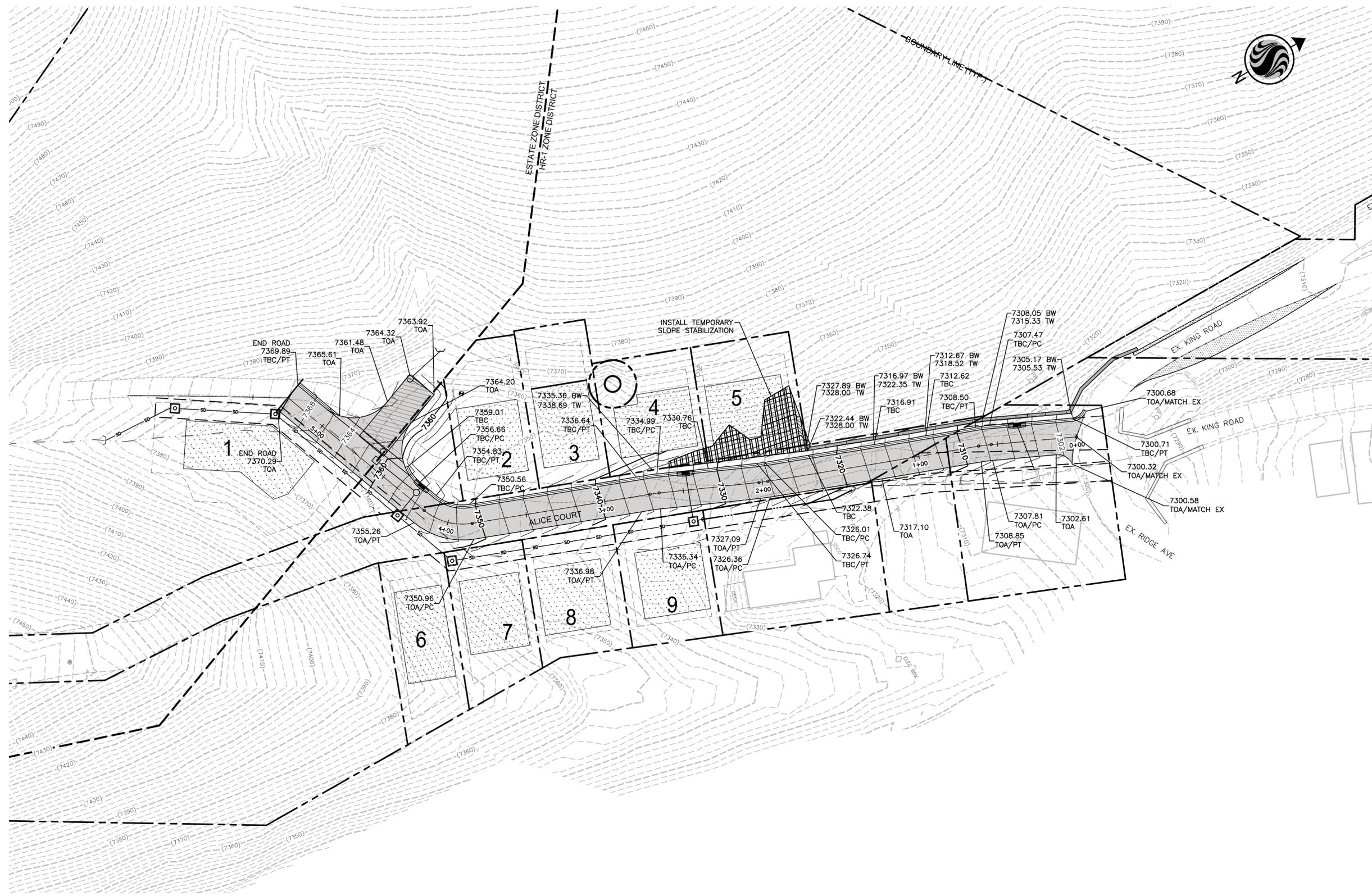
1. TEMPORARY RETAINING WALLS SHALL BE CONSTRUCTED ACROSS FUTURE DRIVEWAYS. FUTURE DRIVEWAYS AND FUTURE RETAINING WALLS N.I.C.
