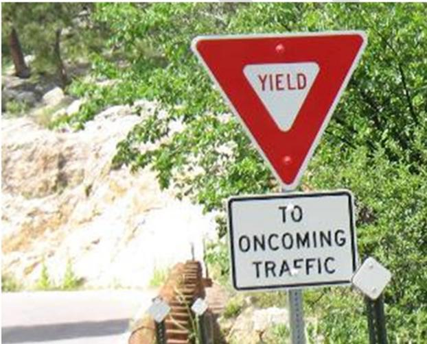
Figure 7: Example of Yield Sign and Supplementary Plaque – Pine Hill Road near Harrisburg, PA
