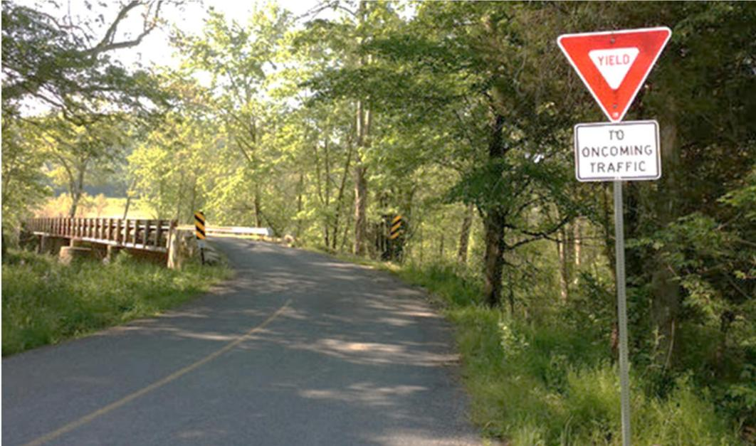
Figure 8: Example of Yield Sign and Supplementary Plaque – Hana Highway in Maui, HI
