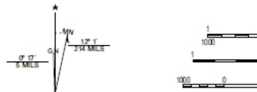
UTM GRID AND 2011 MAGNETIC NORTH DECLINATION AT CENTER OF SHEET
