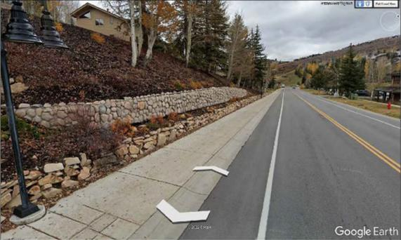
AREA OF CONCERN FOR 12' SIDEWALK DUE TO RETAINING WALL RELOCATION & EXISTING UTILITIES
