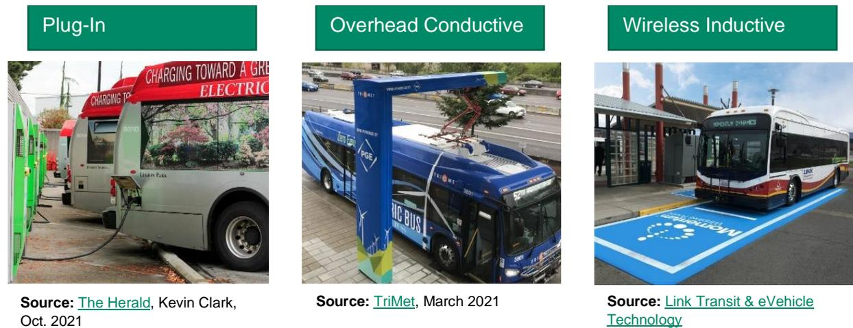
**Plug-in chargers** can be either an ‘All-in-one’ unit with dispensing plug-in cord attached directly to the charger cabinet or a charging cabinet connected to remote plug-in dispensers.
