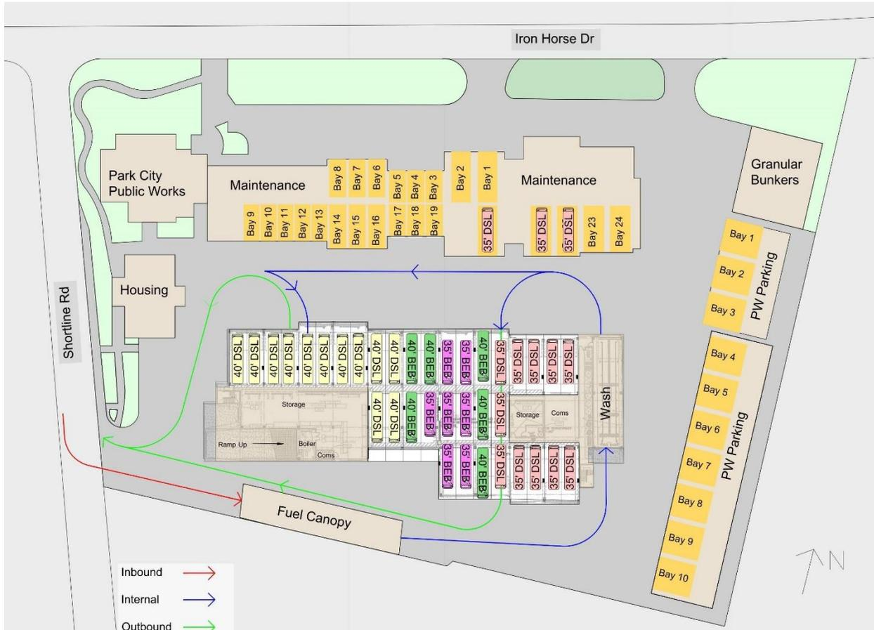
Figure 8: Iron Horse Facility Operations Layout
