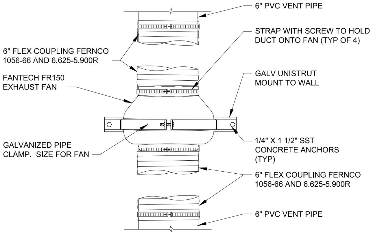
**IN-LINE EXHAUST FAN DETAIL**
