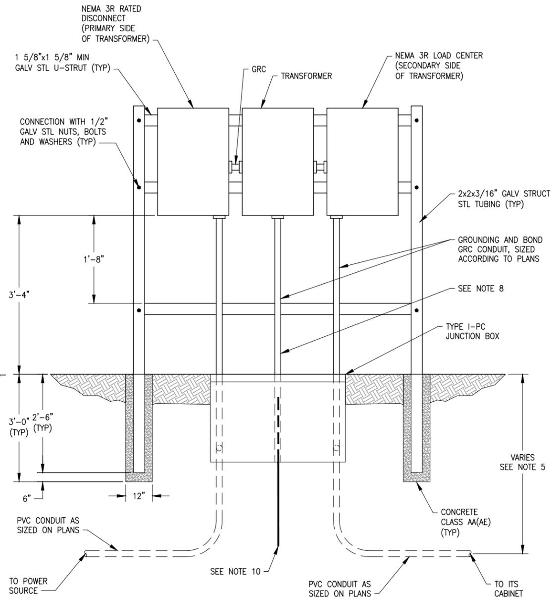
SUPPLEMENTAL DISCONNECT WITH TRANSFORMER FRAME (B)
