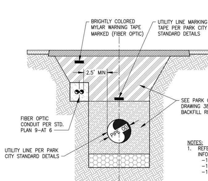
**FIBER OPTIC CONDUIT IN COORDINATION WITH OTHER UTILITY INSTALLATION** (F)
