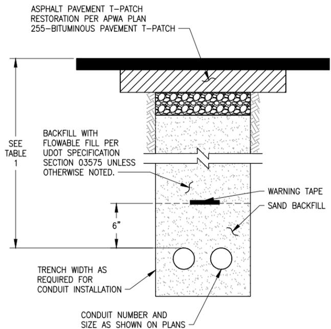
**CONDUIT TRENCHED IN ASPHALT PAVEMENT RESTORED WITH T PATCH** (E)
