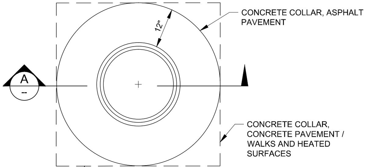
PROVIDE HEATING SYSTEM DISCONNECT AT COLLAR LIMITS. 24" COLLAR REQUIRED FOR 4' AND 5' MANHOLES AND VAULTS
