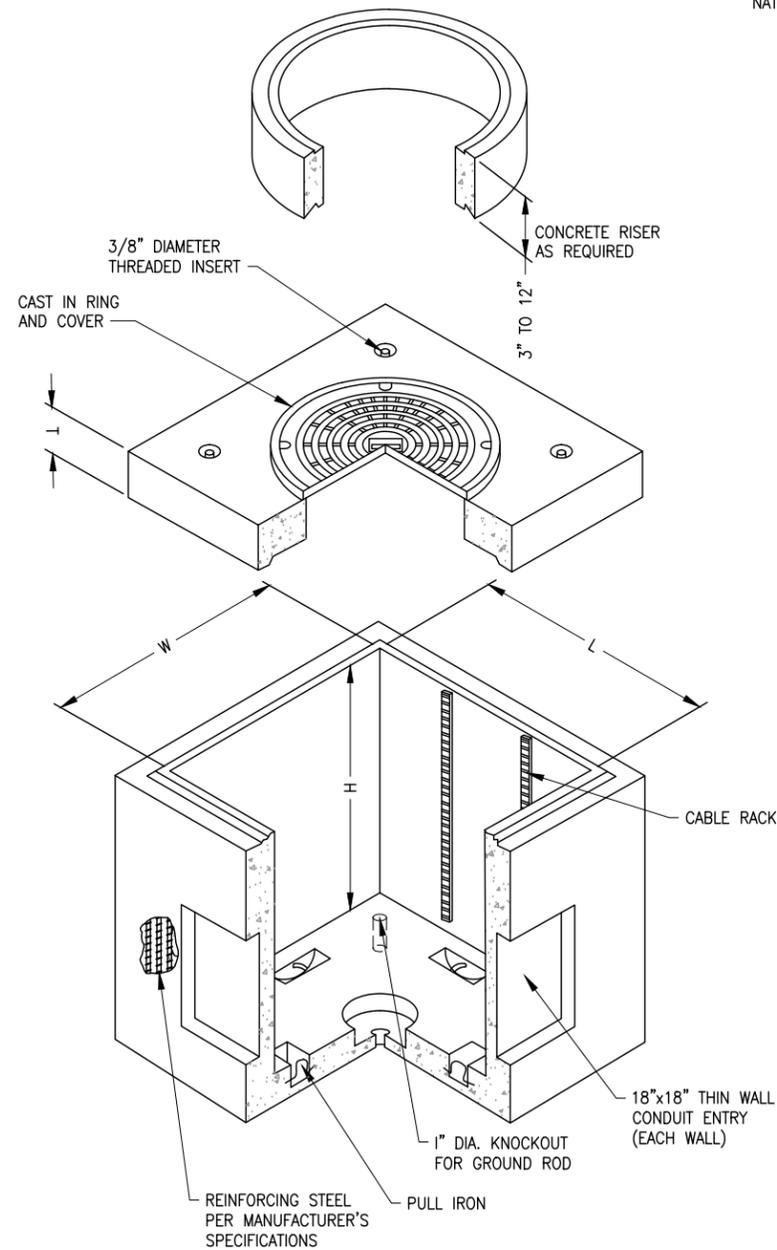
**CONCRETE FIBER VAULT WITH MANHOLE LID**
