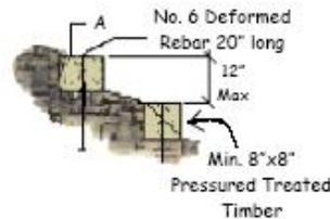
**Stone Stairs**--can be used where trail grades exceed the maximum allowable slopes and where the grade must be gained quickly. Stone stairs should be built with the intent that intensive use should not impact the stairs in the slightest.
