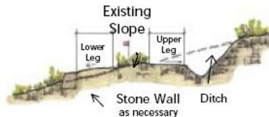
Locate switchbacks where natural barriers exist; installing physical or visual barriers or providing sufficient separation between the switchbacks all help to discourage crosscutting. If crosscutting cannot be discouraged through design or construction then the installation of stairs or relocation of the trail should be considered.
