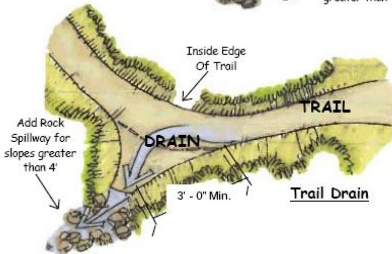
**Trail Drain:** Use where trail construction requires drainage such as along long and/or steep vertical ascents. Do not use where established drainageways exist. They are best if located at low points or bends in trail. Transition from Trail to drain may require 6' at low points. 6' transition will be required up to normal trail.
