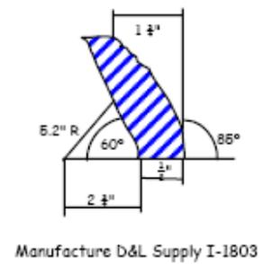
**Water bar:** Water bars will likely need to be installed at regular intervals on soft surface trails that are steeper than a 5% gradient for more than five vertical feet. Rubber water bars should be used since they are the safest for multiple use trails, also construction is more economical, faster and easier than other construction methods.
