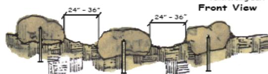
**Note:** Size of barrier stones shall be approximately 14"-24" in height, width and length. Minimum dimensions shall not be less than 12" for height and width and 18" for length.
