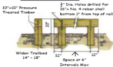
Use where motorized access could be a problem, such as at trailheads, where trails intersect or cross streets and where trails parallel roads at points where access is likely.
