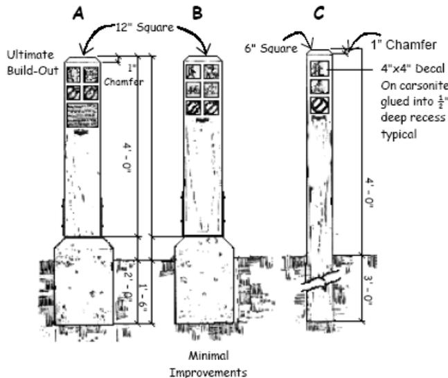
**Attachment Systems:** Signs should be attached to wood posts with 2" diameter galvanized carriage bolts in a minimum of two locations per post.
