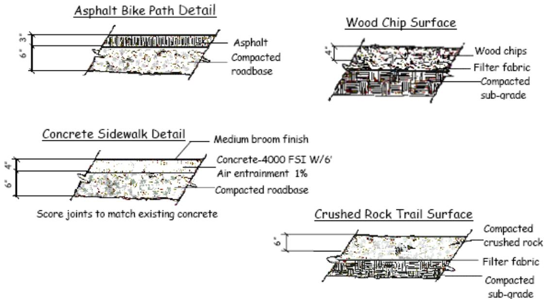
**NOTE:** The crushed rock surfacing may be substituted with 2" of compacted dolomite limestone as per the specification.
