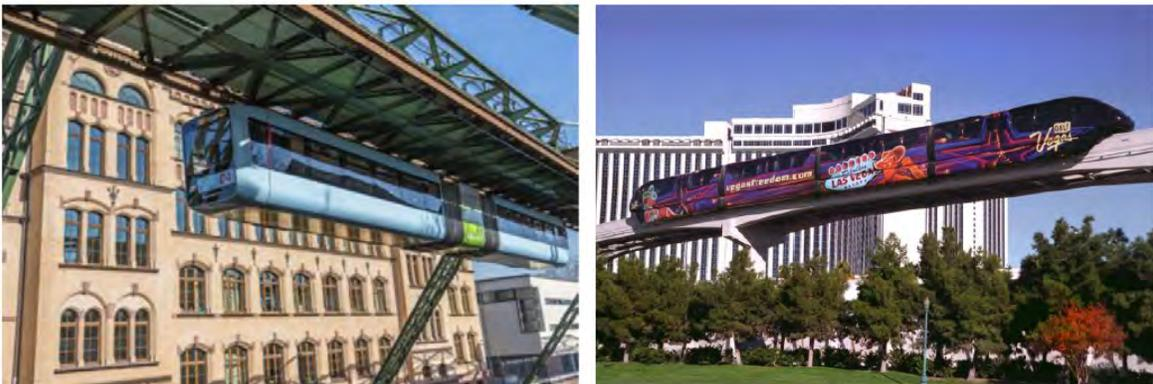
**Figure 2. Suspended Monorail Wuppertal, Germany (left) and Straddle Monorail Las Vegas, United States (right)**
