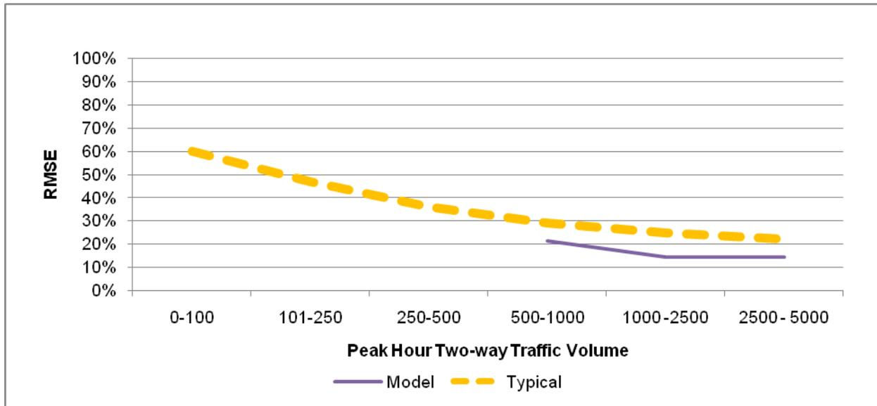
A comparison between the link level FHWA link level guidelines and the calibrated model are shown in Table 8 using estimated peak hour volumes from the ADT guidelines. The shoulder season model results show that 88% of links meet the guideline while 100% of high-ski season meet the guidelines. The correlation coefficient for the shoulder season falls within the national standard of 0.89.
