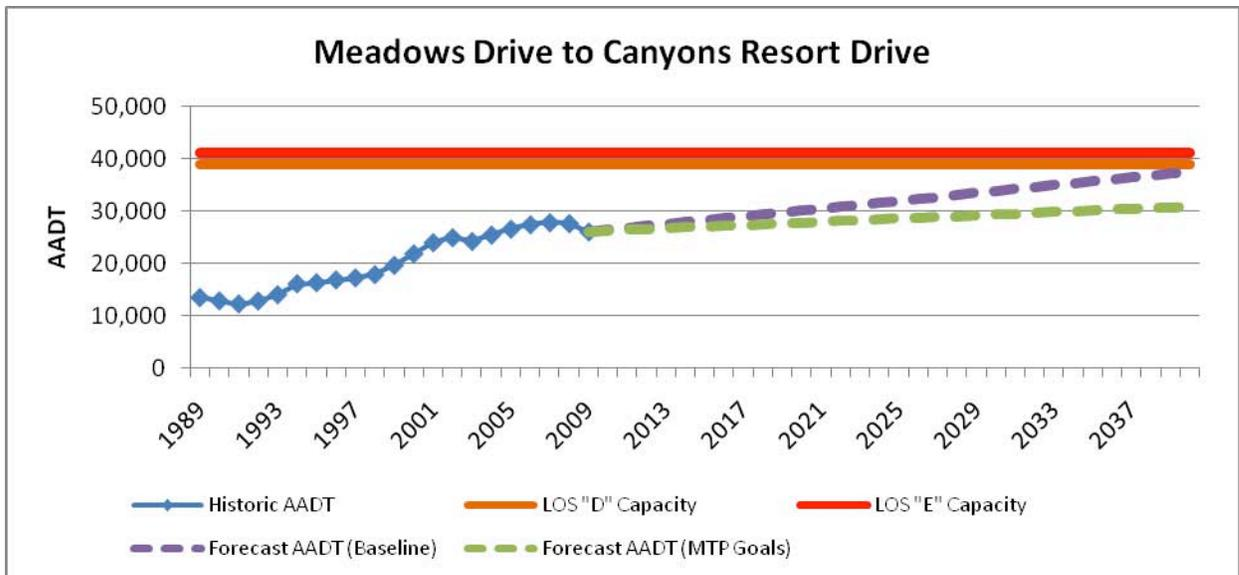
Figure 5 shows traffic volume and screening level of service for the entire corridor SR-224 for existing and future conditions. For the corridor analysis, it was assumed SR-224 would be widened from I-80 to the Canyons as planned in phase II (2021-2030) of the UDOT LRTP.
