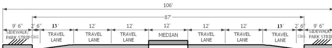
Assuming the 106 foot right-of-way and symmetrical widening of SR-224, Table 10 provides the number of parcels and structures that potentially would be impacted by widening SR-224. The impacts are concentrated between Kearns Boulevard and Deer Valley Drive/Empire Ave. Figure 14 illustrates which parcels might potentially be effected.
