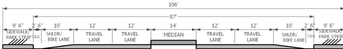
**Figure 28: Modified Seven-Lane Cross-section, 106' Right-of-Way**
