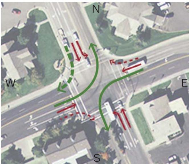
Figure 15. Right Turn Overlap Diagram
